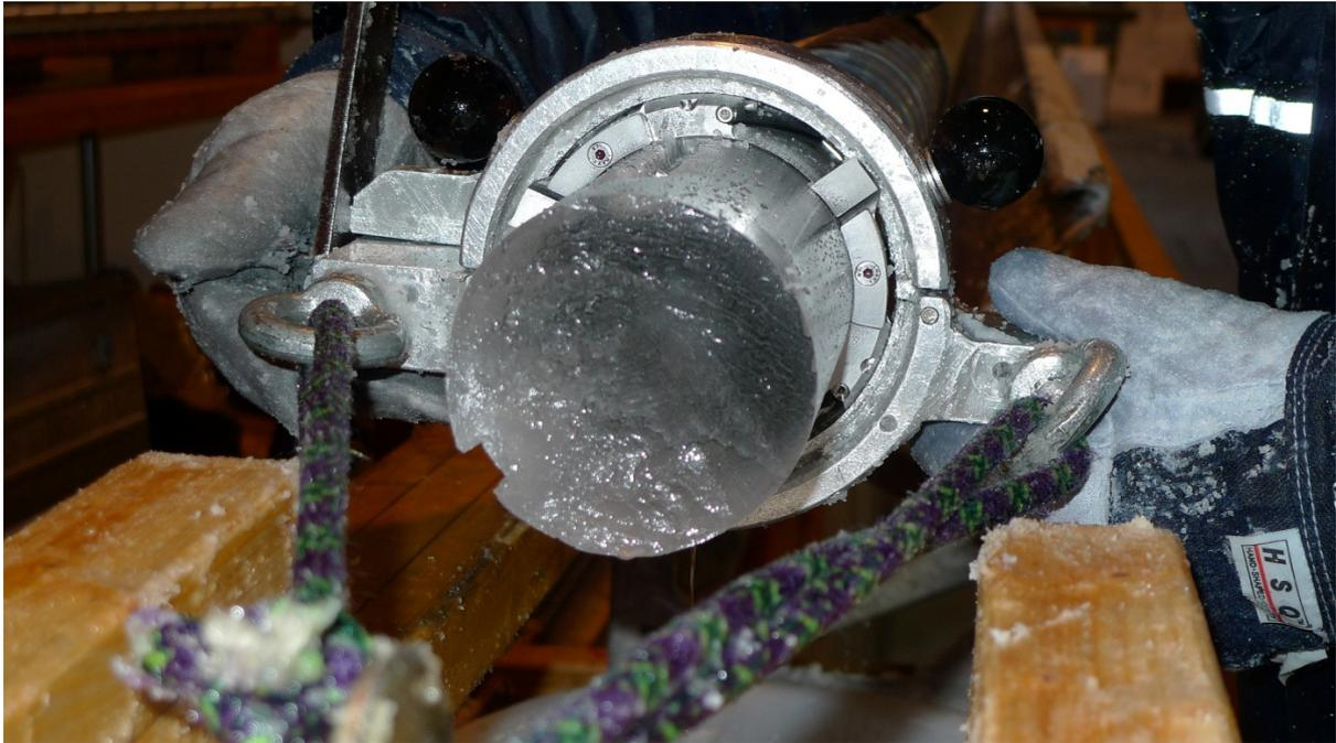
Eisbohrkern. Foto: Sepp Kipfstuhl; NEEM ice core drilling project, <http://www.neem.ku.dk>.
